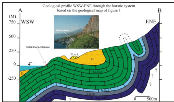
Figure 2. Geological profile WSW-ENE through the karstic system based on the geological map of figure 1 and photo of "Selinitza's" entrance.
