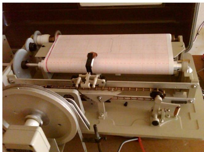
Fig. 1. Water level measuring devices in the J-17 well.
