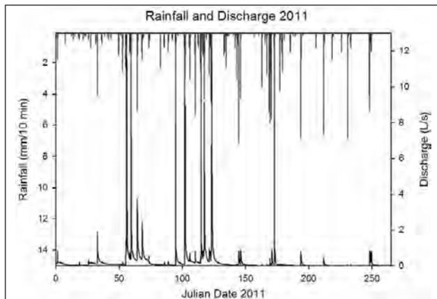
Figure 5. Example of discharge response in WF1 during storm events from 2011.
