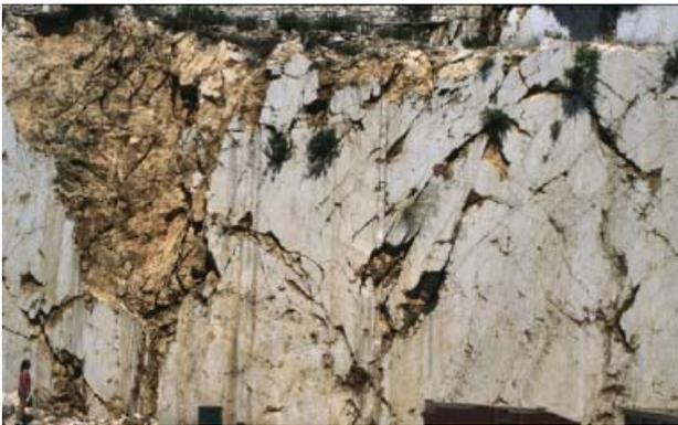
**Fig. 10.** A sawn face 10 m high on a construction site sections limestone just below rockhead in a karst of class kIV in northwestern Sicily. Small caves and dissolutional-opened fissures are mainly aligned on dipping fractures, and a buried sinkhole is exposed on the left after its fill has been removed. Note person at lower left for scale.
